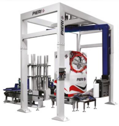
SILVER GO CAD and SILVER FAST CAD are PIERI's arm wrapping machines with Cardboard corners Applicator Device. The automatic device CAD permits the protection of the four angles of the product and it allows the application of the cardboard corners through a vacuum system installed on the four mechanical arms. The CAD device, composed by 8 corner warehouses, can manage different corner dimensions.
