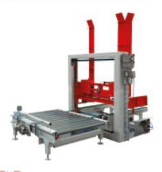
The EMPTY PALLET DISPENSER satisfies on one side the requirement of depositing empty pallets and on the other feeding pallets for the production line. The operator will deposit empty pallets in the warehouse and the automatic device, equipped with conveyors, will dispense the pallets to the production line. The capacity of the system is up to 15 pallets.
