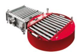
The TURNTABLE STATION and ROLLER/CHAIN EXCHANGER enable the palletized loads to change direction. The turntable station consists of a roller conveyors or chain conveyors able to rotate on its axis allowing the 90° exit of the palletized loads without changing the feed front side. While, the roller/chain exchanger combines the characteristics of roller and chain conveyors in the same position allowing the 90° exit of the palletized loads with changing the feed front side.
